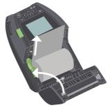
4. Pull the tags through so that it they are exposed when the printer cover is closed, then close the printer cover.
