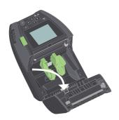
1. Open the printer top cover by pressing the green release button, and lifting open the cover.
