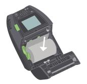
Insert the media between the label holders as shown. Take care to ensure the tags are oriented correctly.
