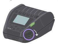
1. Open the interface cover on the side of the printer
